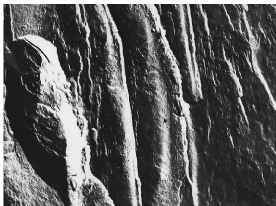
Fig. 3. Transmission electron micrograph of the four-component sample 3 made by freeze-fractured technique at magnification of 18,000 \times .
